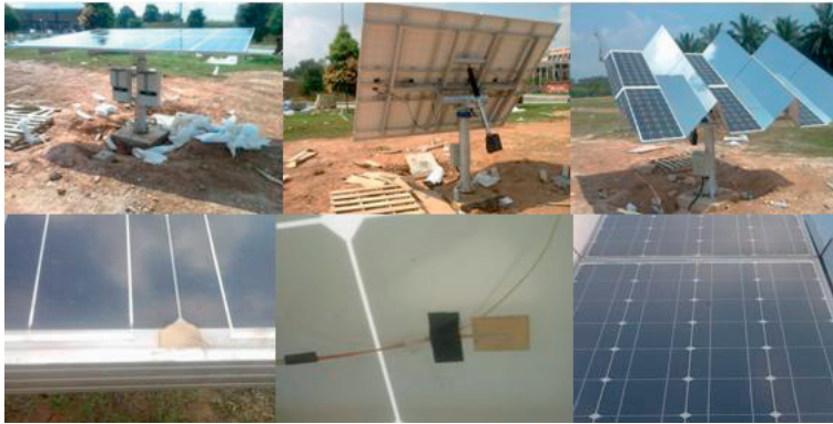
Figure 1: Site setup of multiple PV array configurations with thermocouple sensor
