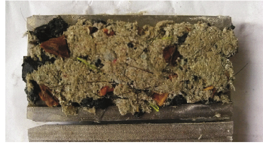
Fig. 3. Plugging zone formed with the three types of LCMs.
