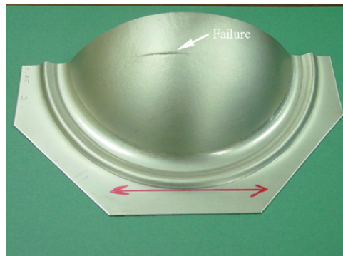
Fig. 11. (a) Simulation using yield function with constant coefficients. (b) Simulation using evolutionary yield function. (c) Experiment (half of bulged specimen) at strain rate \dot{\epsilon} = 0.05 \text{ s}^{-1} .
