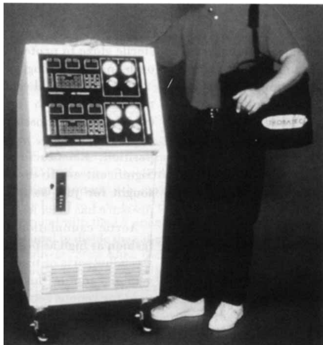
Fig V. To the right of the patient is the dual-drive console contrasting, with the portable TLC-II (Thoratec) slung from the patient's left shoulder. The portable driver has biventricular pumping capabilities and provides for improved patient mobility.
