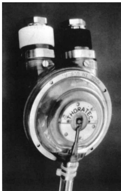
Fig III. The prosthetic ventricle is shown with the black colletnut on inflow housing and white colletnut on outflow housing. The fill switch can be seen in the middle of the housing of the ventricle and the electrical and pneumatic connection at the bottom.
