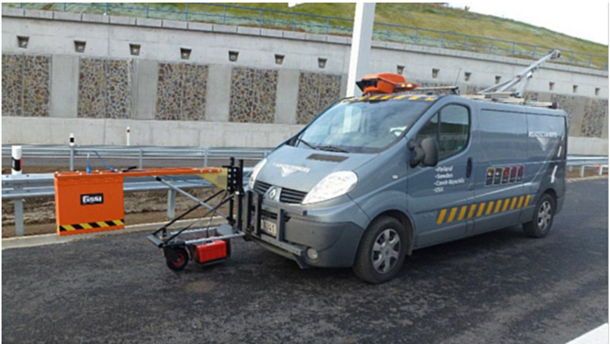
Fig. 2. Road Doctor Survey Vehicle used in the project data collection. The system consists of 1. GPR system with 2.0 GHz horn antenna and 400 MHz ground coupled antenna, 2. CamLink System for digital video recording, 3. 3D accelerometer and 4. 2D laser scanner.
