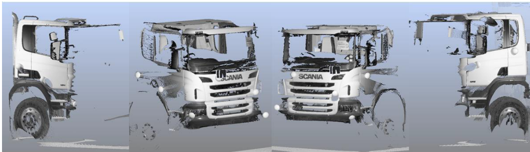
Fig. 2. Example exterior scans for the Scania P cab vehicle. The reference spheres used to aid alignment of the scans are visible in the images.
