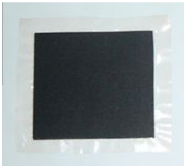
Figure 1 Membrane electrode assembly.
