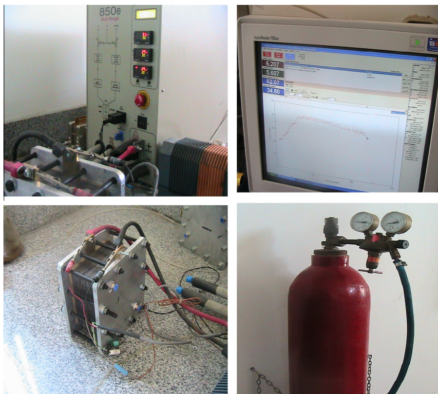
Figure 2 Fuel cell stack test station.
