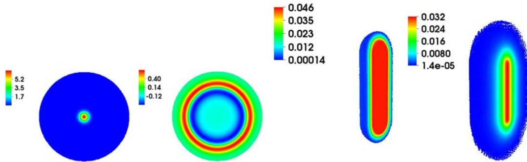
Figure 2: 2D simulation of liquid disk with free surface (two left images). 3D simulation of gas expansion into vacuum (two right images show pressure distribution).
