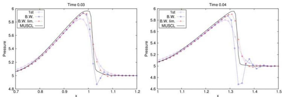
Figure 1: Gaussian pressure wave propagation with periodic boundaries at time 0.03 (left) and 0.04 (right). Coarse-resolution simulations results were used to illustrate the behavior qualitatively.
