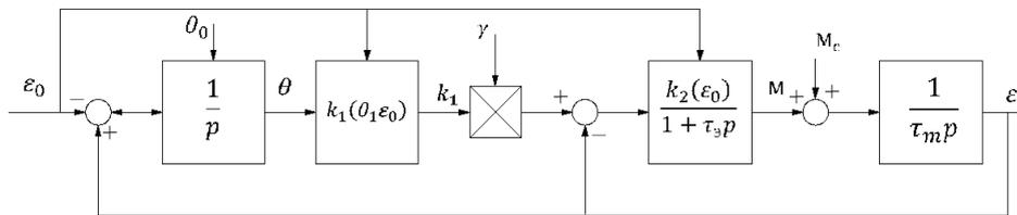
Fig. 1. Block scheme of PMSM in the synchronous rotation mode.
