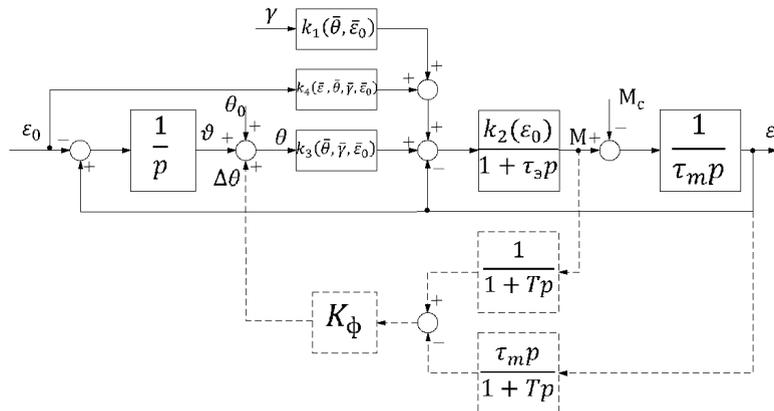
Fig. 2. Linearized block scheme of PMSM in the synchronous rotation mode.
