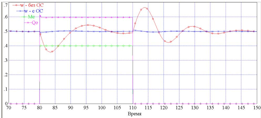
Fig. 3. The results of permanent-magnet synchronous motor operation modelling in a synchronous mode.
