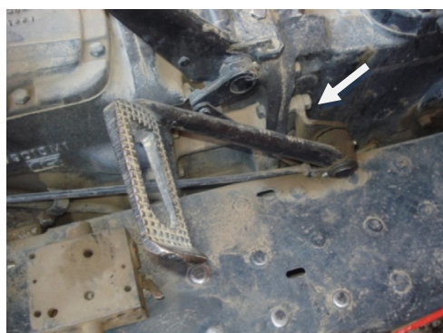
Fig. 5 – The pivot pin of the clutch release linkage and the way in which is currently attached to the gearbox casing of MF285 tractor.
