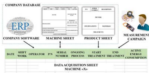
Fig. 2 – Data acquisition sheet
