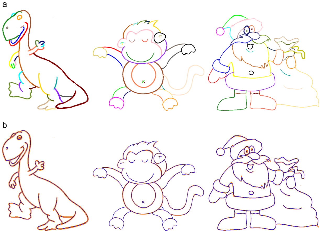
Fig. 16. Segmentation and vectorization of several simple line drawing images. We use different color to render extracted line Stokes. (a) Results of segmentation; (b) fitting B-spline curves as a vectorization of the image. The number of data points (pixels) are 10,637, 9436 and 5066 from left to right respectively. (For interpretation of the references to color in this figure caption, the reader is referred to the web version of this paper.)
