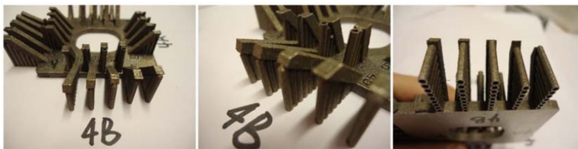
Fig. 13. Macrographs of tube support structure with diameter of 2 mm.
