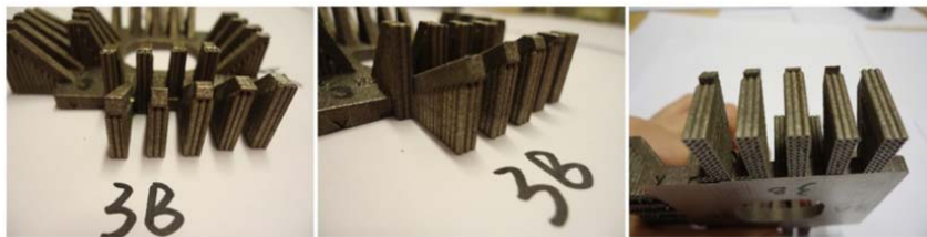
Fig. 12. Macrographs of tube support structure with diameter of 1.3 mm.
