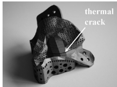
Fig. 3. Cracks caused by thermal stresses. (Kruth et al., 2012).
