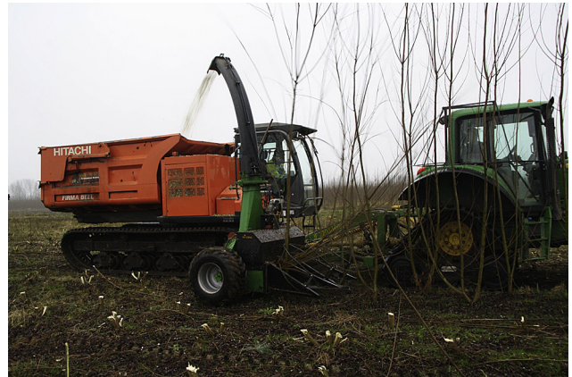
Fig. 2 – View of the tractor-pulled cut-and-chip harvester operating at the short rotation woody crop operating on willows.
