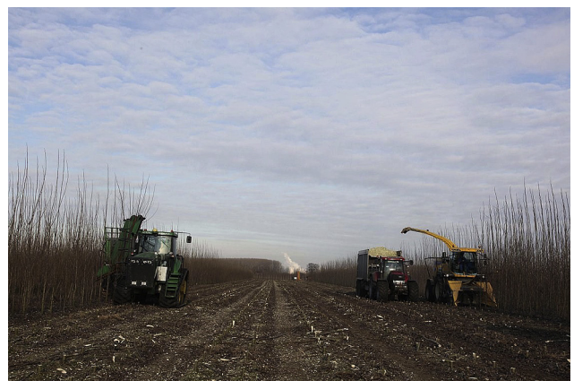
Fig. 3 – View of the tractor-pulled whole stem harvester (on the left) and the self-propelled cut-and-chip harvester with the trailer–tractor combination (on the right) operating at the same short rotation woody crop poplar plantation.
