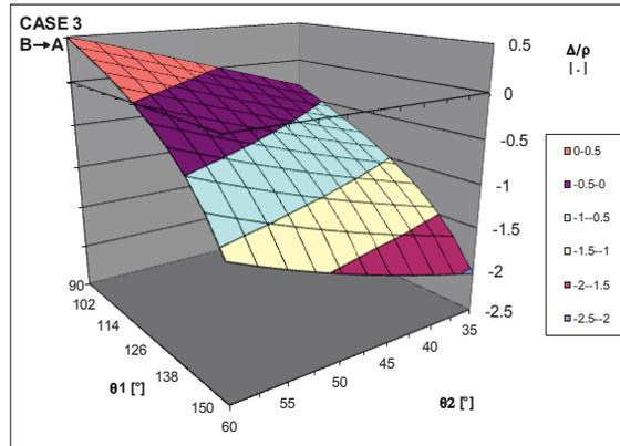
Fig. 11. Trend of  $\Delta\rho$  by varying  $\theta_2$  and  $\theta_1$  for Case 3 (B→A)
