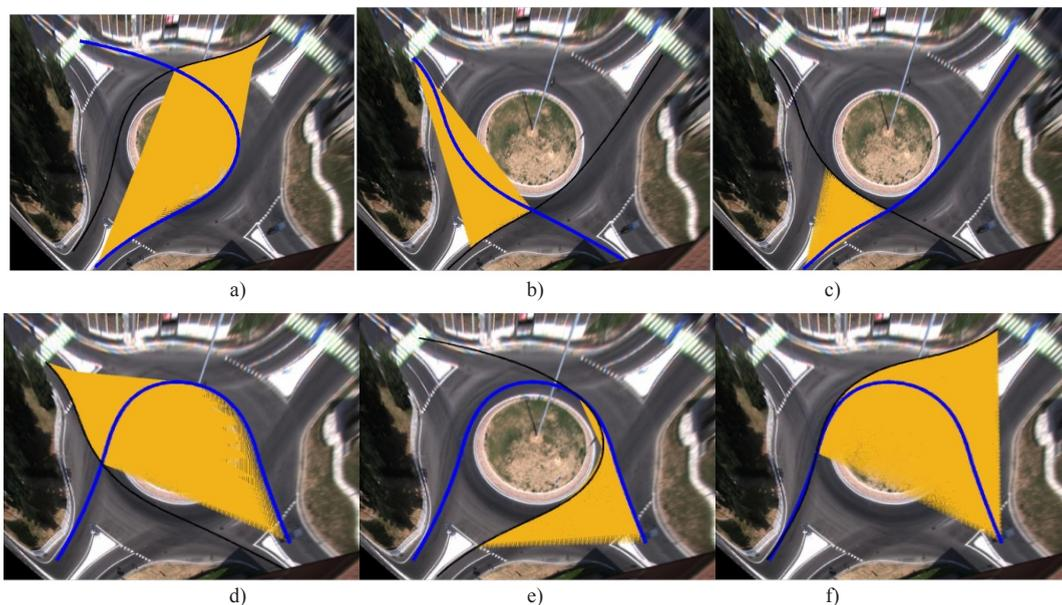
Fig. 13. Crossing of two trajectories (A has the gray line and B the black line) and the area (gray hatched) where  $\Delta$  is positive: a) Case 2, A→B; b and c) The effect on  $\Delta$  by changing the reciprocal position of A and B for the same trajectories Case 3, A→B (b), and Case 3, B→A (c); d, e, and f) The effect on  $\Delta$  by changing the crossing trajectory of vehicle B, Case 2, A→B (d), Case 3, B→A (e), and Case 3, A→B (f)
