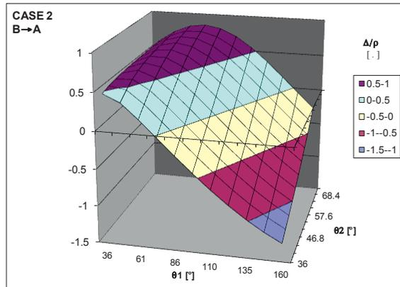
Fig. 8. Trend of  $\Delta/\rho$  by varying  $\theta_2$  and  $\theta_1$  for Case 2 (B→A)
