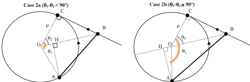
Fig. 6. Reference scheme for computation of relative distance between two vehicles (A e B) in Case 2 with  $(\theta_1-\theta_2)<90^\circ$  (a) and with  $(\theta_1-\theta_2)\geq 90^\circ$  (b)
