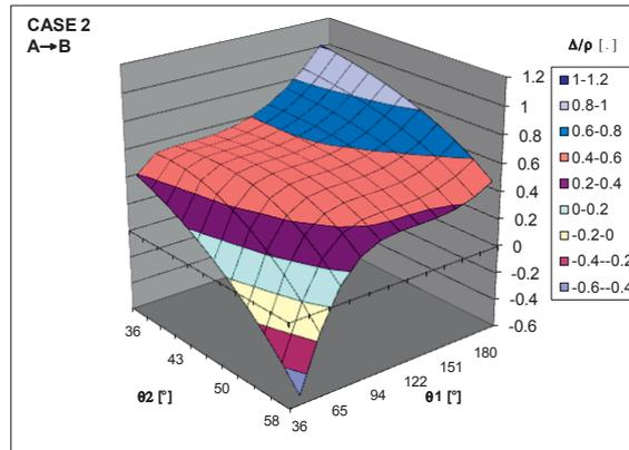
Fig. 7. Trend of  $\Delta/\rho$  by varying  $\theta_2$  and  $\theta_1$  for Case 2 (A→B)
