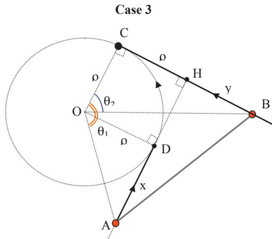
Fig. 9. Reference scheme for computation of the relative distance between vehicles (A and B) for Case 3 (both vehicles are entering)
