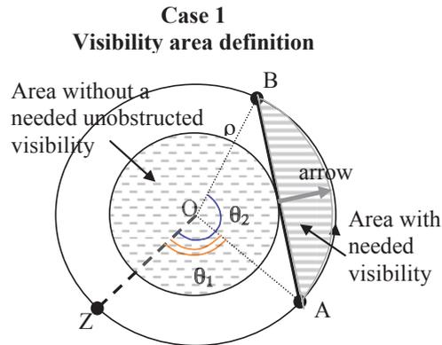
Fig. 5. Visibility arrow (the gray arrow) and area (of central island or circulating roadway) without visibility
