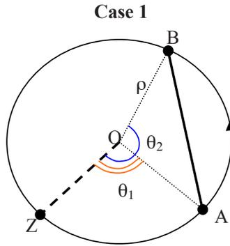
Fig. 3. Reference scheme for computing relative distances between two vehicles (A and B) for case 1 (both vehicles are circulating in the circulating roadway)
