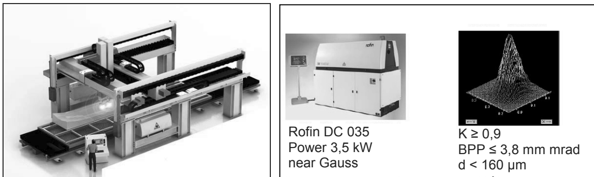
Figure 2: Large welding machine for industry-orientated welding and the integrated CO 2 -laser (12)
