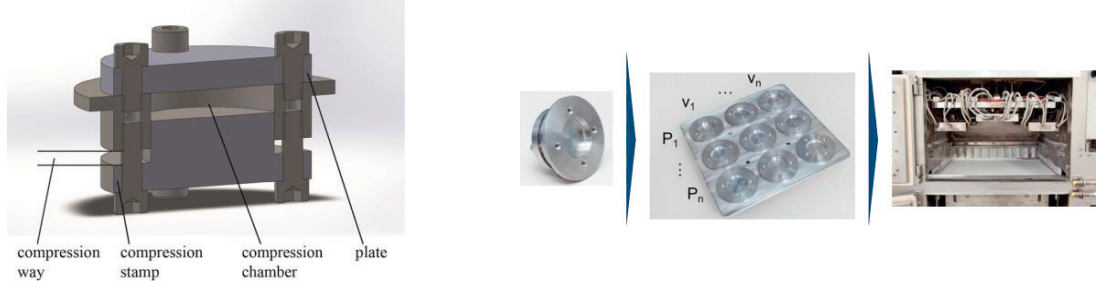
Fig. 4. Small building chamber (left); placed small building chambers in the SLM-system (right)
