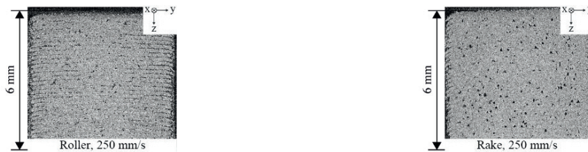
Fig. 12. CT-Scans for cubic specimens exposed with varying heating rates at constant coating speed
