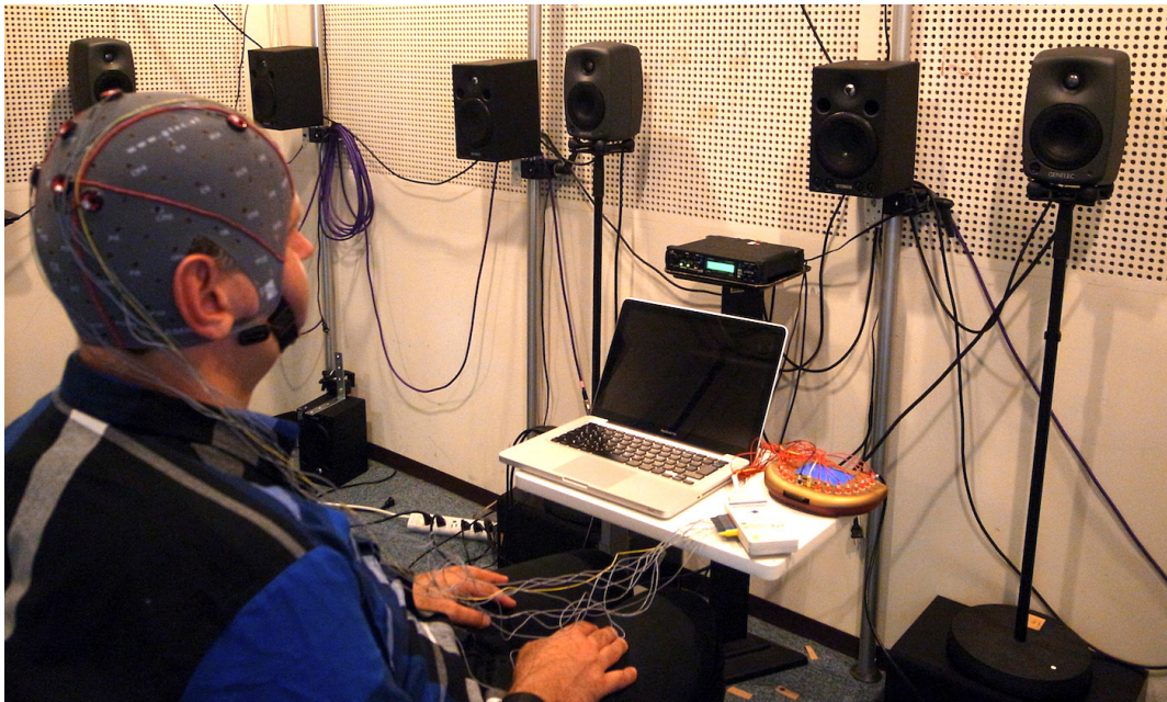
Fig. 3. The experiment environment in which the spatial auditory BCI-speller paradigm trials were conducted using the BCI2000 software [9] to capture and classify the brainwaves. The spatial acousting environment was created using the loudspeakers depicted in the photograph and managed with a MAX programme developed in-house. The BCI user depicted is wearing an EEG cap with active electrodes g.LADYbird by g.tec Medical Instruments GmbH, Austria, connected to an amplifier vAmp by Brain Products GmbH, Germany.
