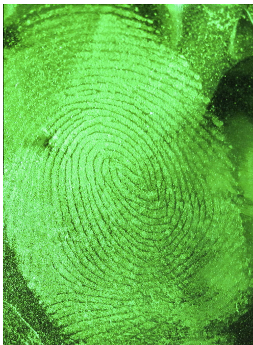
Figure 7 Latent fingerprint developed on aluminum foil exposed to 200 °C with formulation A.
