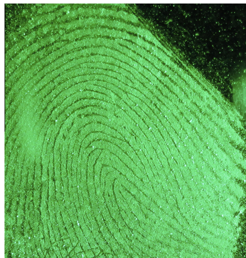
Figure 6 Latent fingerprint developed on glass exposed to 300 °C with formulation A.
