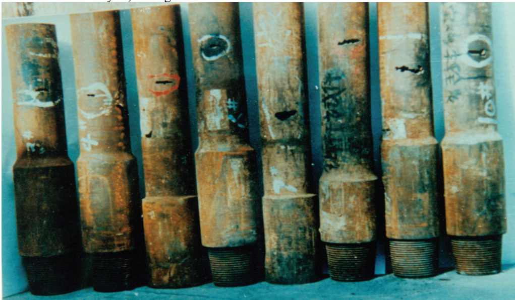
Fig.1 Washout morphology of drill pipe in transition zone
