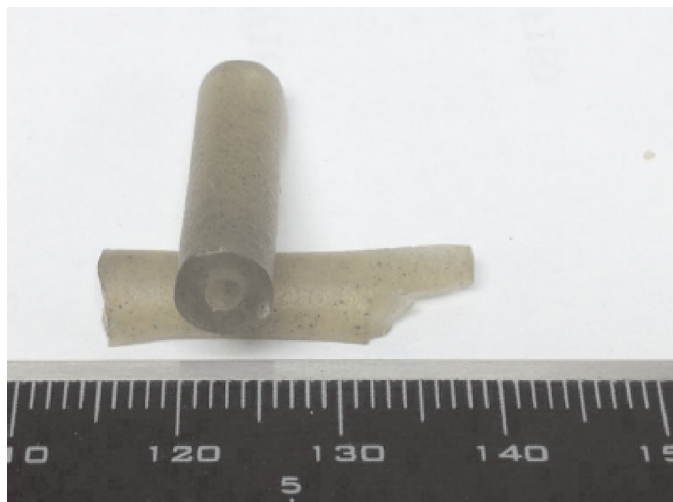
Fig. 2. RPD380 without BN-single perf grain used in erosion testing.
