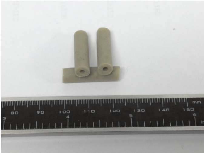
Fig. 3. BN-RPD380 (US patent pending) single perf grains used in erosion testing.
