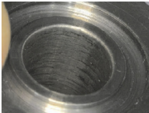
(b) RPD380 P – flow exit end – cleaned after 3 shots
