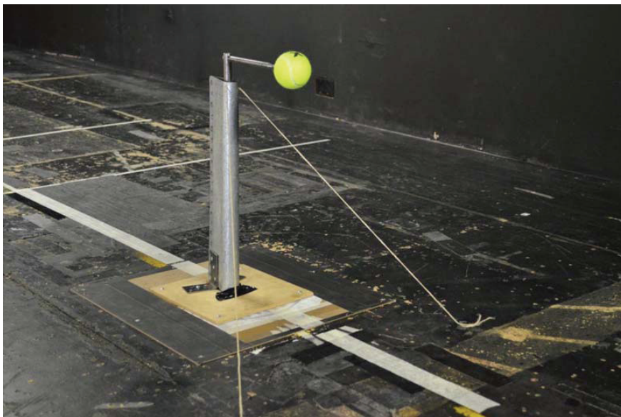
Fig. 1. Side view of horizontal setup of sting and tennis ball
