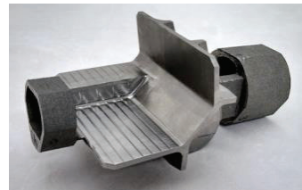
Figure 9: Hinge part after machining prior to removing sacrificial fixtures
