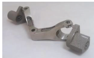
Figure 11: Finished suspension part prior to removing sacrificial machining fixtures.
