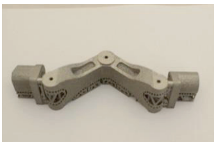
Figure 10: Suspension part with sacrificial fixtures, support structures for AM process and 1.0 mm machining allowance
