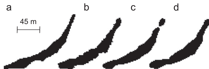
Fig. 2. Example of a data template. Cross-sections of (a) the training image, (b) cleaned maximum, (c) cleaned median and (d) cleaned minimum simulated models of the deposit (in terms of volume).
