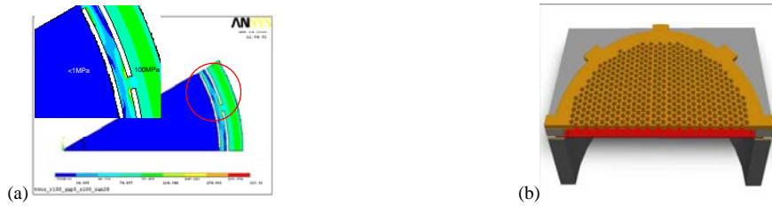
Fig.1 (a) 1/12 simply Ring type FEM stress relaxing design (b) half model cross section
