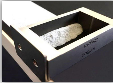
Fig. 3. Film applicator with deposited PP powder layer.
