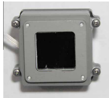
Fig. 3 Digital sun sensor.
