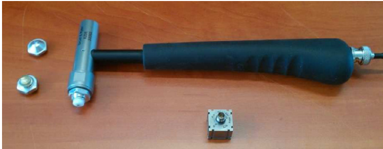
Fig. 2 Modal hammer with heads of various stiffness and triaxial accelerometer
