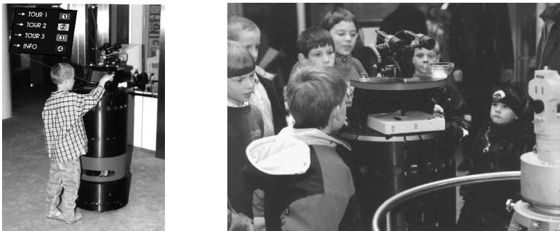
Fig. 23. On-board interface of the tour-guide robot. The users were required to press the buttons right from the display to choose between different options (left image). During the tour the robot used its camera to point to the exhibits. It showed text and graphics on its display and played pre-recorded sounds from CD to explain the exhibits (right image).
