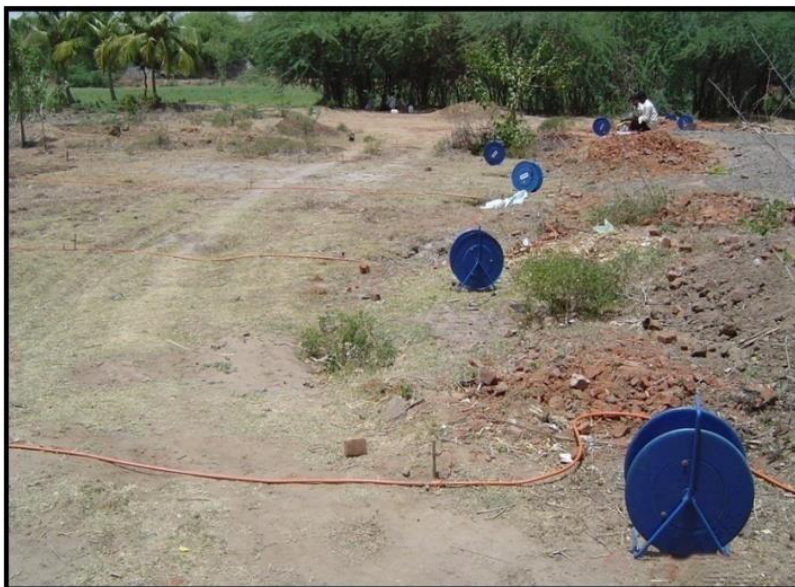
Fig. 4. Multi-electrode winch set-up
