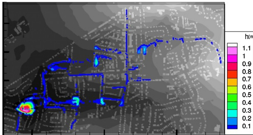
Fig. 1. Flood map of Central model (West Garforth case study area) showing water depth (h).
