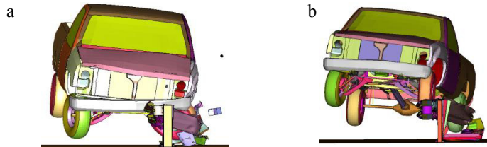
Fig. 14. (a) Actual U shaped guardrail; (b) Proposed absorber.
