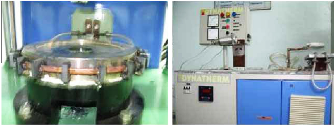
Figure 1 Induction furnace developed to draw the materials at elevated temperature.
