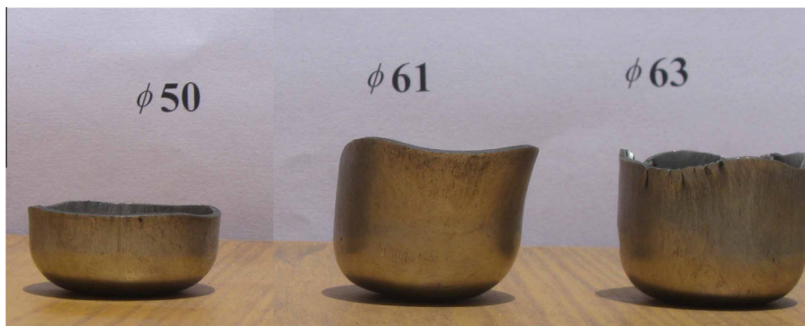
Figure 4 Drawn cups of Al IS 737 alloy at 200 °C.
