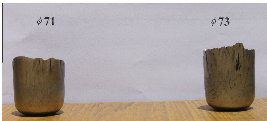
Figure 5 Drawn cups of Al IS 737 alloy at 350 °C.
