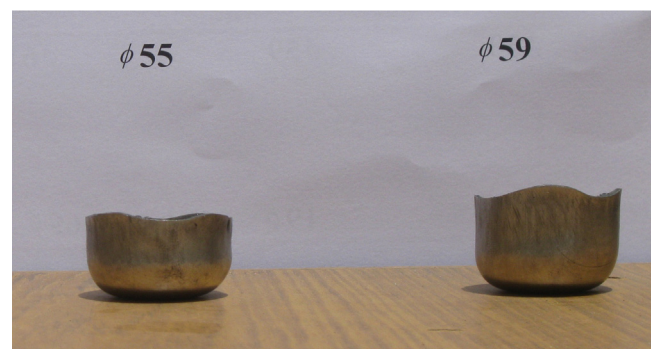
Figure 3 Drawn cups of Al IS 737 alloy at room temperature.
