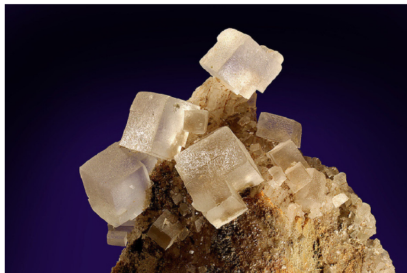
Fig. 1. The cubic habit of a natural sample of Halite (Wieliczka, Poland). Photo: J.M. García-Ruiz.
