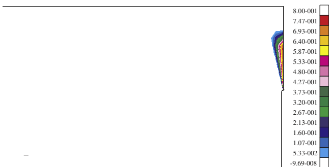
Fig. 13. Contour plot of damage variable \chi corresponding to centerline displacement of 0.0008 mm.
