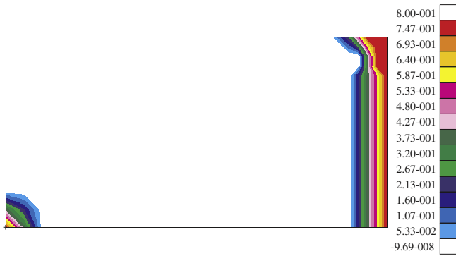
Fig. 11. Contour plot of damage variable \chi in the TPB (un-notched) specimen at applied displacement of u_y = 0.012 mm.
