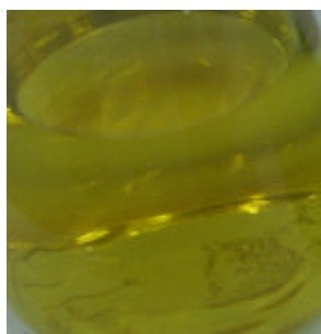
Fig. 2. Silver colloid prepared in aqueous solution using sodium borohydride as a reducing agent
