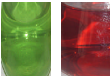
Fig. 8. Observed colors of silver colloids prepared using PVA as stabilizer, silver content: 500
