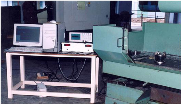
Fig. 1 – Experimental setup used for drilling operation.
