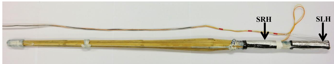
Fig. 2. Top view of Shinai instrumented with sensors for the right (SRH) and left hand (SLH).
