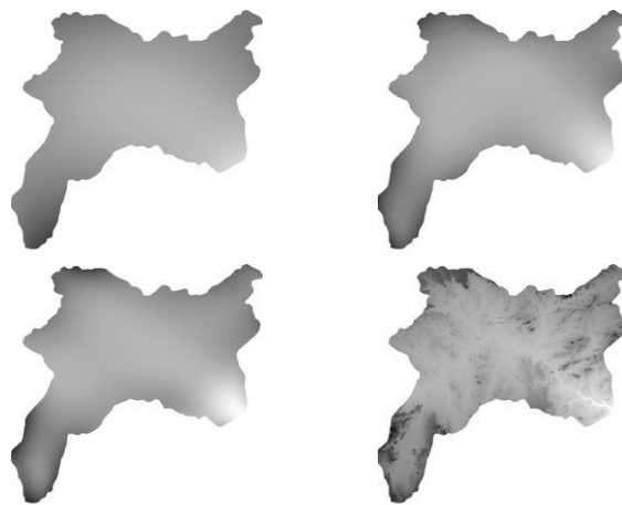
Figure 3: Gray tones landform attributes representation of São Francisco river valley region for polynomial degrees 2, 4, 6 and 20.
