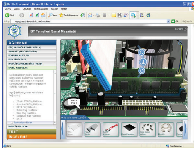
Figure 2. Simulator Laboratory Application (Installing the motherboard PATA Cable)
