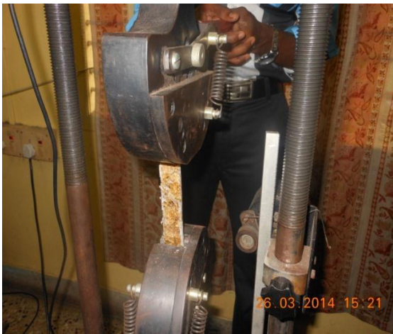
Fig. 4 UTM machine Sample loaded condition for tensile testing
