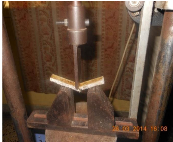
Fig. 5 UTM machine Sample loaded condition for Flexural testing.
