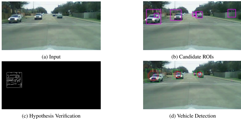
Fig. 1: Proposed vision-based vehicle detection system
