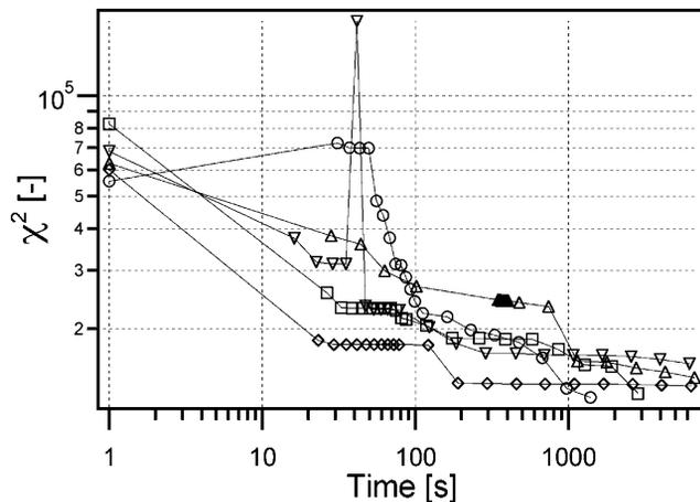
FIGURE 8 Evolution of the least-square estimate  $\chi^2$  during the optimization using different strategies: full guess ( $\nabla$ ), image average ( $\circ$ ), division ( $\Delta$ ), segmentation ( $\circ$ ), and quadrant average ( $\square$ ).
