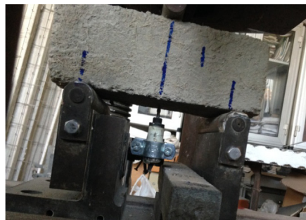
(b) LVDT test set-up
