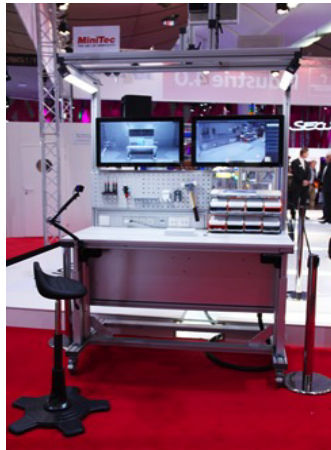
Fig. 2. Business Card Holder's Manual Assembly Workstation ©SmartFactory KL
