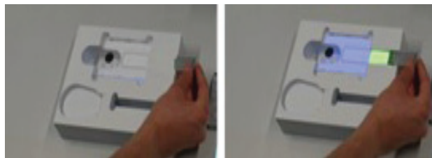
Fig. 1. Traditional Manual Assembly vs. Assisted Manual Assembly ©SmartFactory KL
