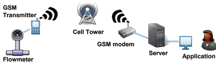
Fig. 2. Schematic of Instrumentation and Server System.
