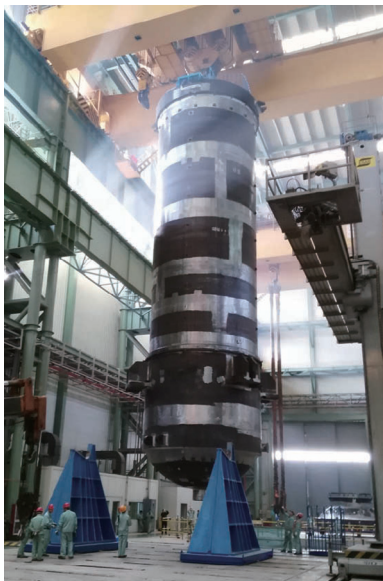
Fig. 4. Manufacture of the HTR-PM reactor pressure vessels by the Shanghai Electric Corporation; status as of September 2015.
