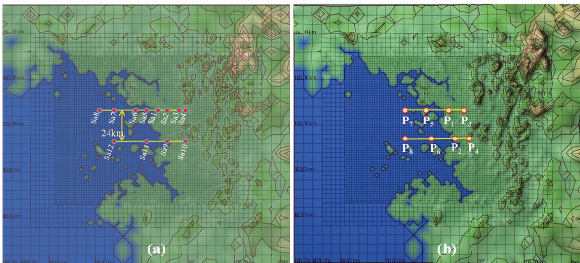
Figure 5. (a) Sa1-Sa12 are the sampling sites of the wind vector and temperature, and (b) P1-P8 are the representation of point sources where puffs are released continuously from 65 m high and 6 m diameter stacks.
