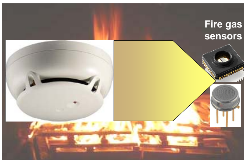
Fig. 3: Illustration of the concept of combination between smoke detectors and gas sensors for false alarm elimination
