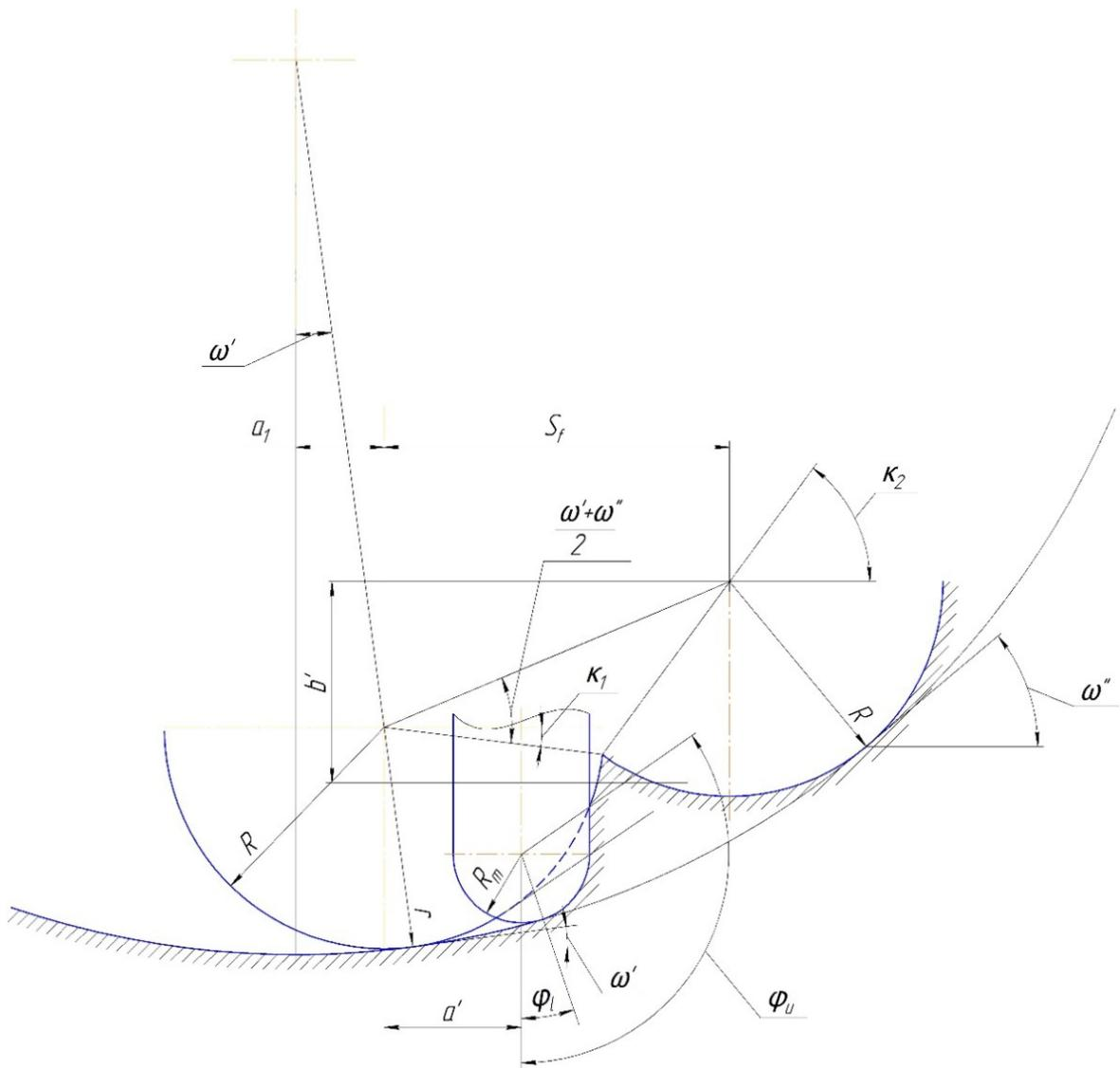
Fig. 3. Geometrical parameters of machining of a concave surface.
