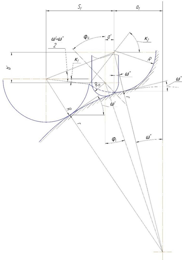
Fig. 2. Geometrical parameters of machining of a convex surface.
