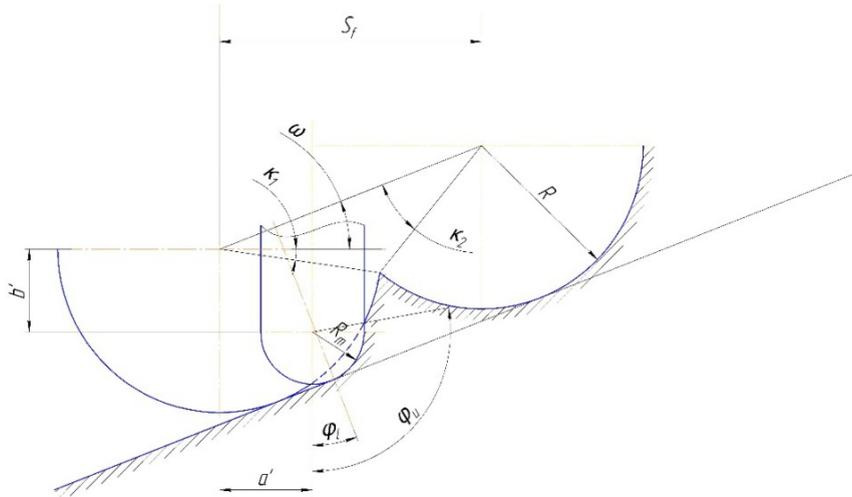
Fig. 1. Geometrical parameters of machining of a flat surface.
